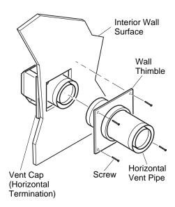
Figure 25 - Connecting Vent Cap with Horizontal Vent Pipe
